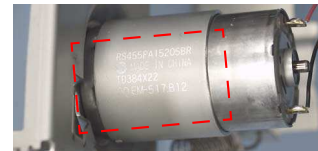
Figure 1-89. Reinstalling the CR Motor
