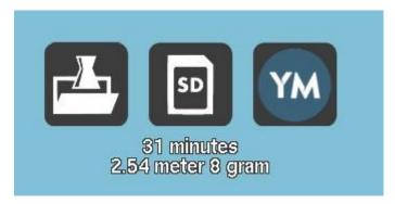
The set of icons located in the upper left corner of the screen is used for reading \*.STL/\*.OBJ files and saving them to the disk or SD card. The estimated time of printing and the length and weight of the waste filament are displayed under the icon.
