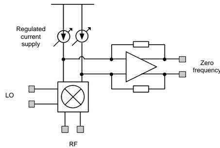
Fig. 7. Mixer output with regulated current supply.
