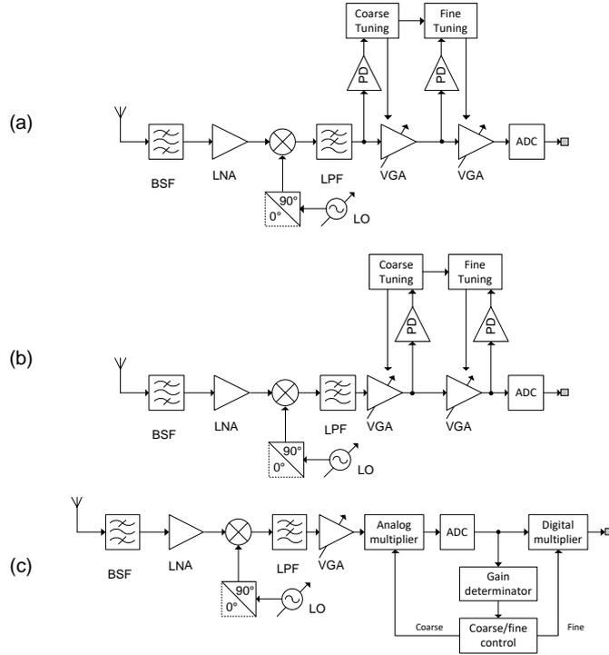
Fig. 9. AGC method, (a) – feedforward, (b) – feedback, (c) – hybrid.
