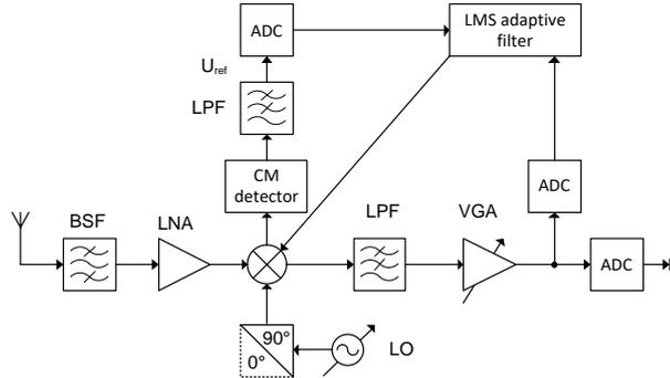
Fig. 6. Receiver adaptive IIP2 feedback calibration method.
