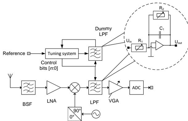
Fig. 8. Indirect LPF corner frequency tuning method.
