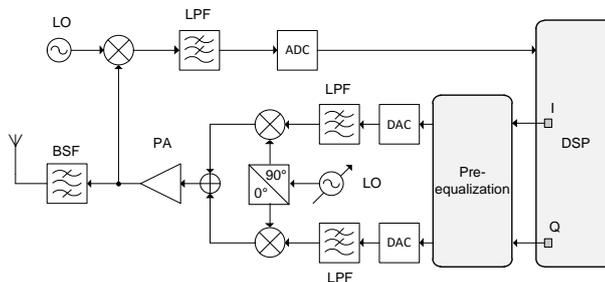
Fig. 4. Transmitter I/Q imbalance feedback calibration method.
