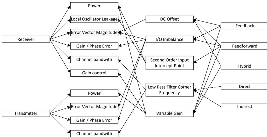
Fig. 1. Relations between transceiver parameters, parameters to be calibrated and calibration methods.
