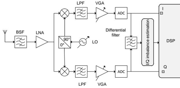
Fig. 5. Receiver I/Q imbalance feedforward calibration method.
