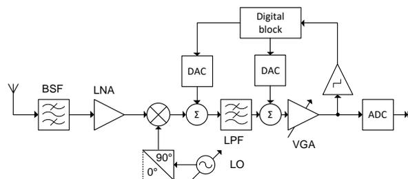
Fig. 3. Receiver VGA two step DC offset cancellation feedback method.
