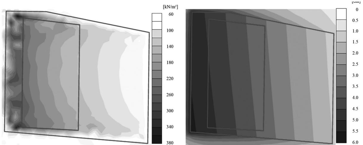
Figure 4. Contact pressure (left) and settlements (right) under the foundation raft
