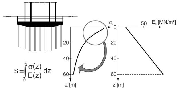
Figure 1. Principle load transfer of a CPRF
