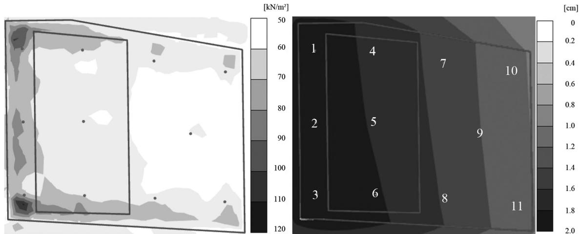
Figure 6. Contact pressure (left) and settlements (right) under the foundation raft of the CPRF
