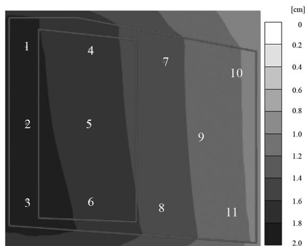
Figure 5. Settlements under the foundation raft of the classic pile foundation
