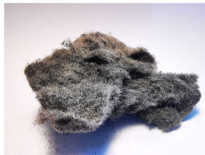
Figure 1. Waste Tyre Textile Fibre used as raw material in the study
