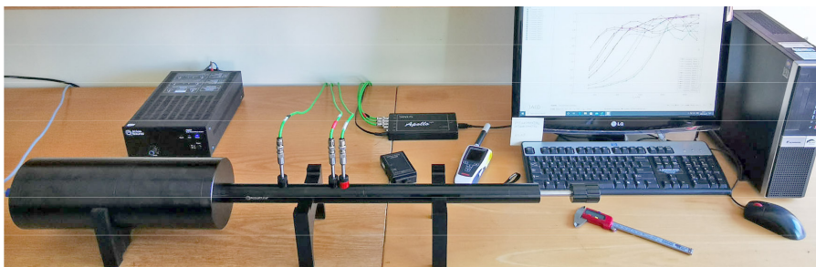
Figure 3. Sound absorption coefficient measurement setup
