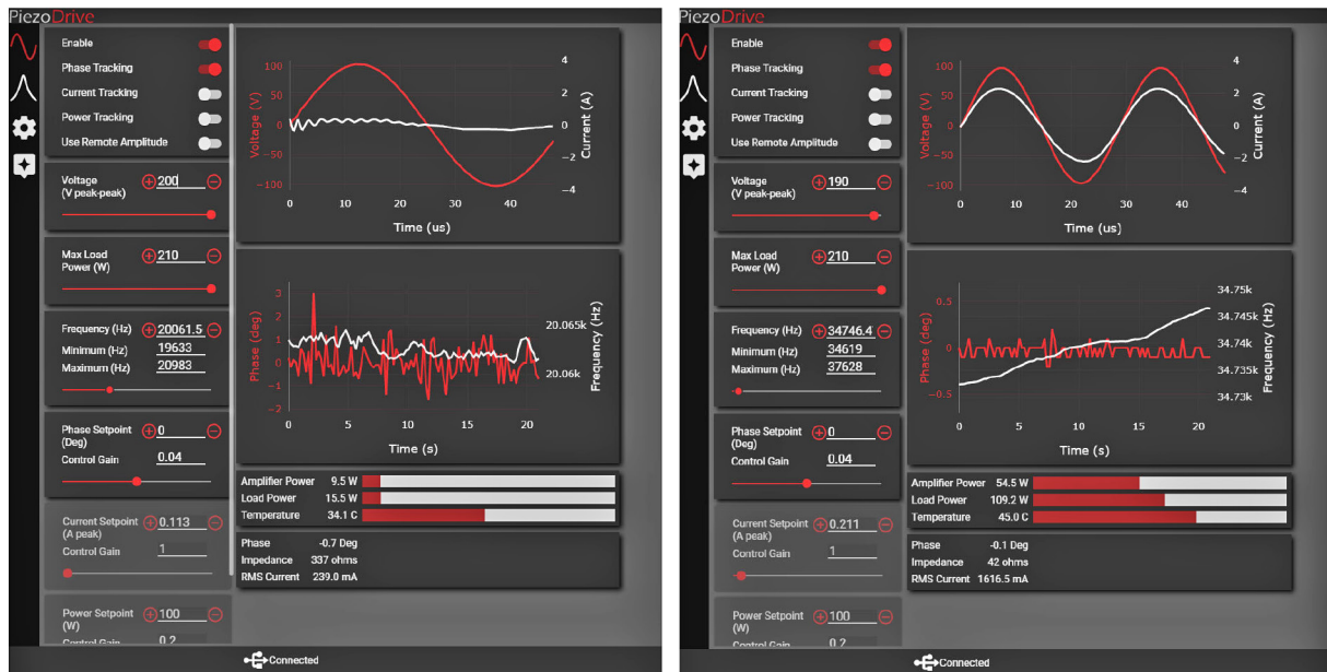
Figure 3. Control parameters of a piezo generator using piezodrive
