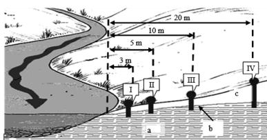
Figure 1. The scheme of multilevel lysimeters places: a – groundwater zone, b – groundwater table, c – aeration zone, I, II, III, IV – multistage lysimetric boreholes
