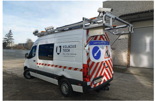
VILNIUS TECH Road Research Institute's mobile laboratory equipped with a laser crack measurement system
